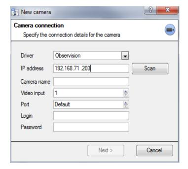
**Driver:** Select the relevant driver for your camera. **IP Address:** Set the IP address of the camera you
